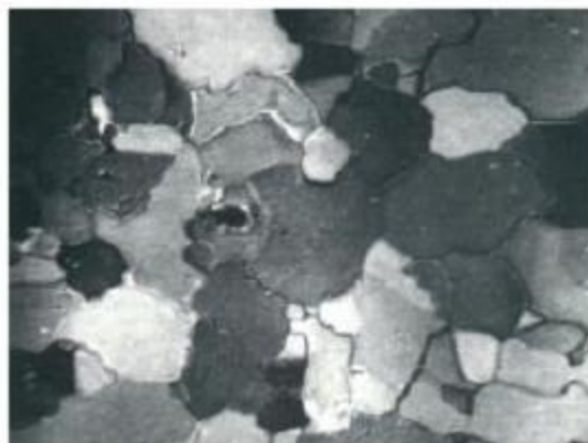
Fig.b: Structure of steel The differences in grey level are caused by the direction dependance of the acoustic velocity. The grain boundaries represent a disturbance in the propagation of the sound waves. Frequency : 1.6 GHz, Image width: 312 \mu m
