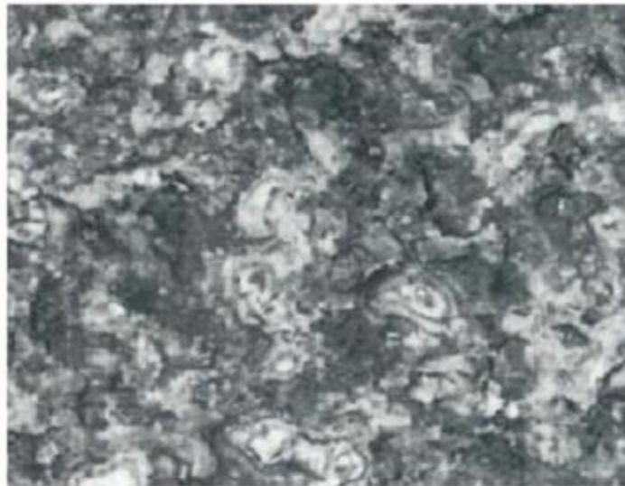
Fig. a: Rough surfaces of a paint layer. The topography is indicated by the formation of contour lines. Inclusions and pores show up clearly due to large differences in their grey levels. Frequency: 400 MHz, Image width: 1 mm
