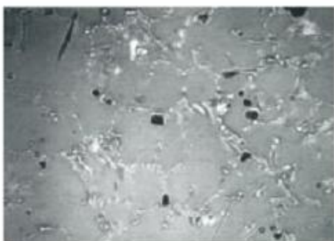
Fig. c: Polished cross section of an alloy with intermetallic deposits and impurities
